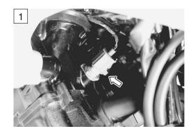
3) Disconnect the ECT sensor coupler and ECM coupler.
