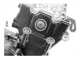
• Apply SUZUKI SUPER GREASE "A" to the O-rings and install them into the cylinder head.
