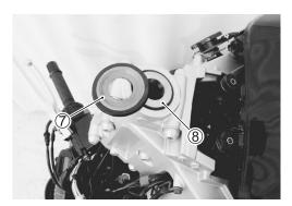
• Remove the steering stem upper bearing inner race 9 and bearing 10.
