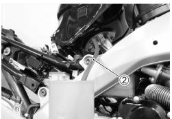
Disconnect the fuel pump lead wire coupler ③.
