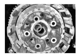
• Install the spring washer seat ⑨ and spring washer ⑩ onto the clutch sleeve hub correctly.
