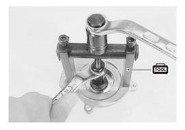
• Remove the oil seal using a suitable bar.
