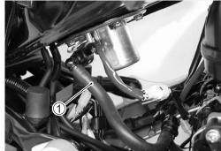
Install the special tools between the fuel tank and fuel delivery pipe.
