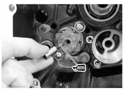
• Install the gearshift shaft assembly ? and washer ? as shown.
