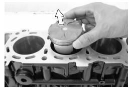
• Remove the piston pin circlip ①.
