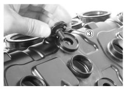
• Tighten the head cover bolts to the specified torque.
