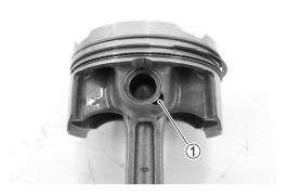
• Separate the piston and conrod by driving out the piston pin. *NOTE:*
