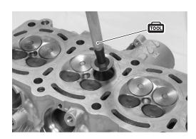
• If the seat width W measured exceeds the standard value or seat width is not uniform, reface the seat using the seat cutter.
