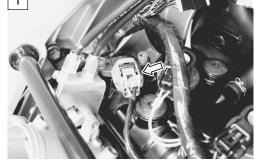
5) Disconnect the CMP sensor coupler and measure the resistance.
