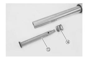
• Pull the inner tube out of the outer tube with light impact.
