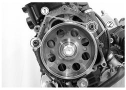
• Install the generator cover and tighten the generator cover bolts to the specified torque.
