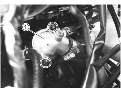
• Pour engine coolant and bleed air from the cooling circuit. (2-17 and -18)
