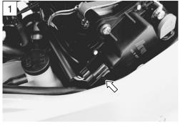
4) Turn the ignition switch to ON to check the STV operation. (STV operating order: Full open  $\rightarrow$  95% open)
