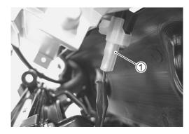
· Test the cooling fan motor for load current with an ammeter connected as shown in the illustration.
